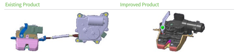
Example of parts integration: Power tailgate latch
